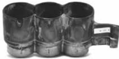
Surface failure in die-casting dies
