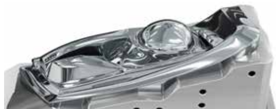
A highly polished mould for production of car headlights.
